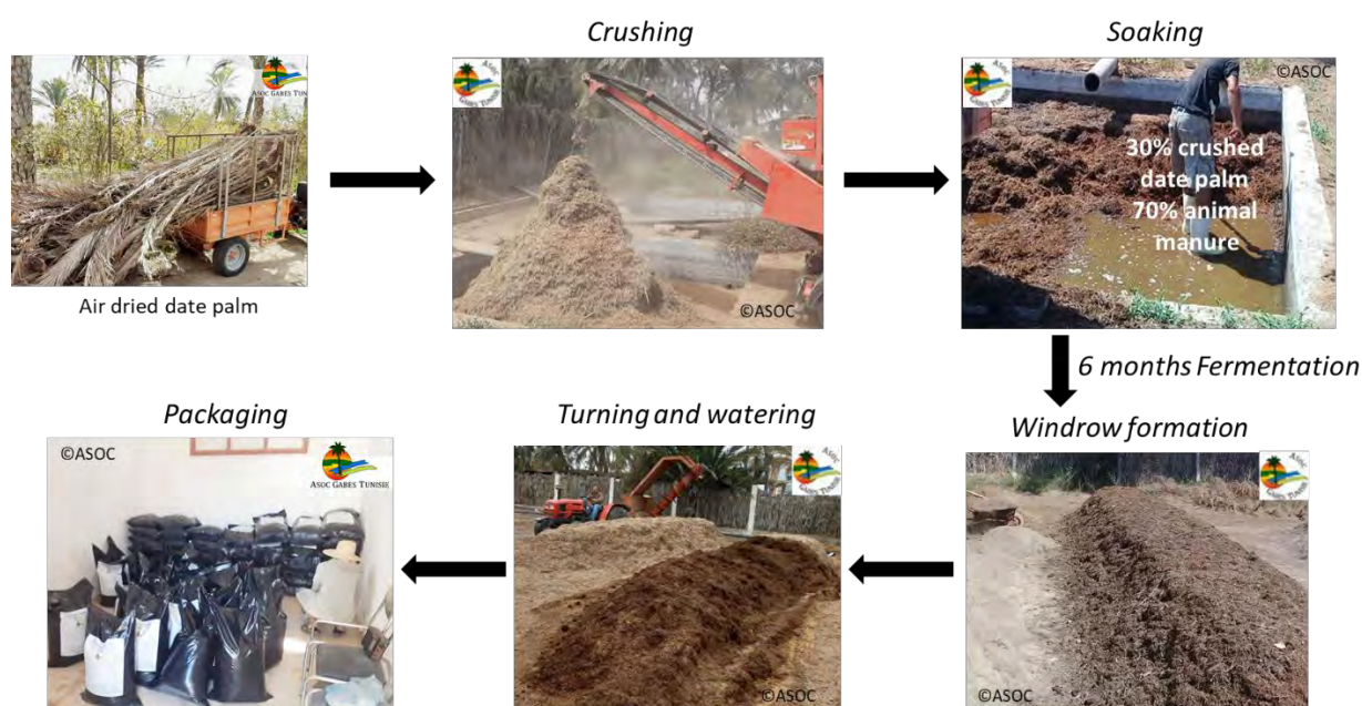
Figure 14: Compost production processes in ASOC, Tunisia
