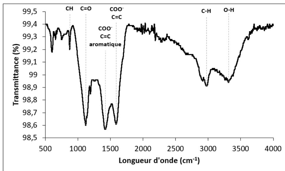
Figure 13 : Fourier Transform Infrared (FTIR) Spectrum of Biochar (Le Guyader et al., 2024)
