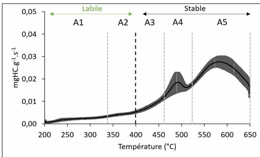
Figure 12 : Thermogram S2 for date palm biochar with temperature limits of pools A1 to A5 defined by Malou et al. (2020). (Le Guyader et al., 2024)
