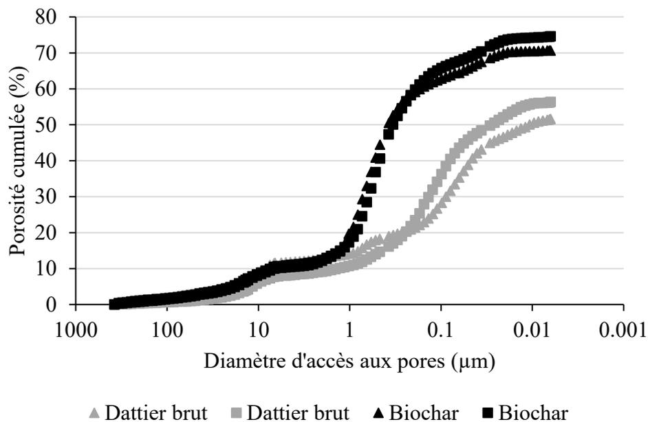
Figure 14 : Cumulative porosity of raw date palm rachis and biochar as a function of pore size determined by mercury intrusion porosimetry. (Le Guyader et al., 2024)
