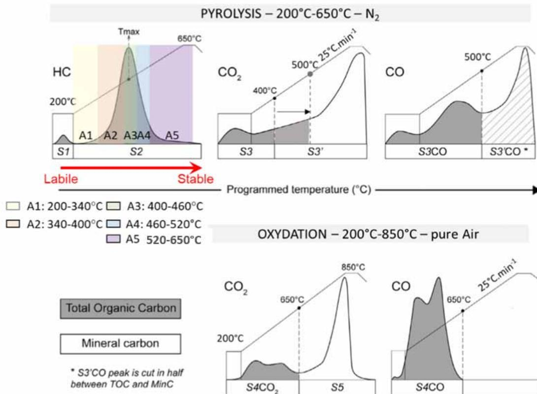
Figure 11 : Principle of Rock-Eval 6 analysis (Le Guyader, 2024, modified from Ducasse et al., 2023).
