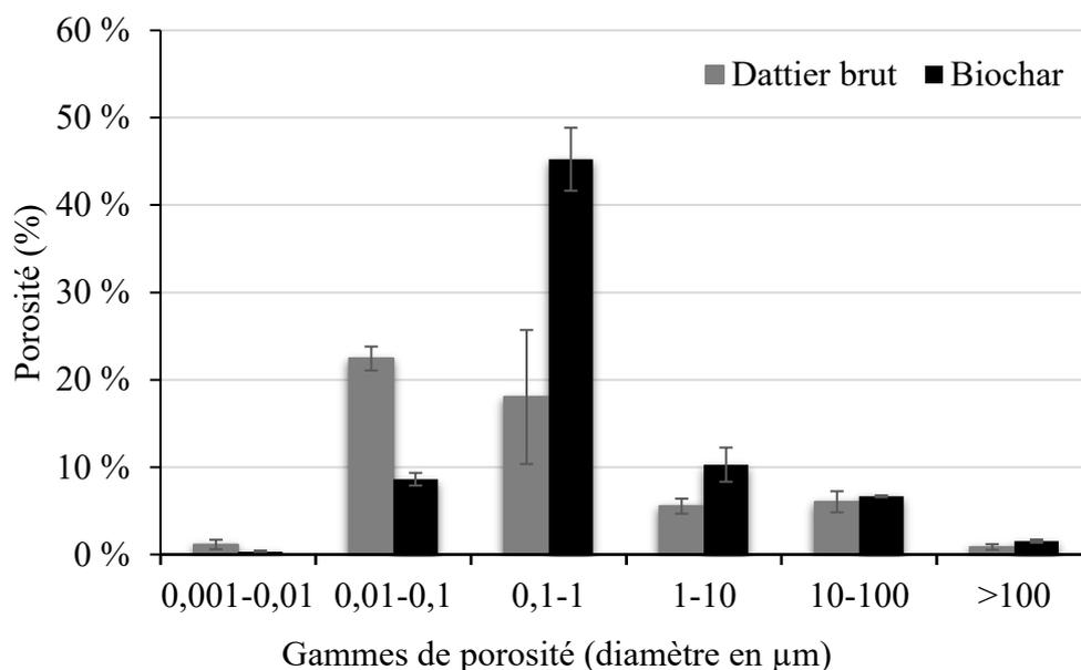
Figure 15 : Distribution of pore size of date palm rachis before and after pyrolysis (Le Guyader et al., 2024)
