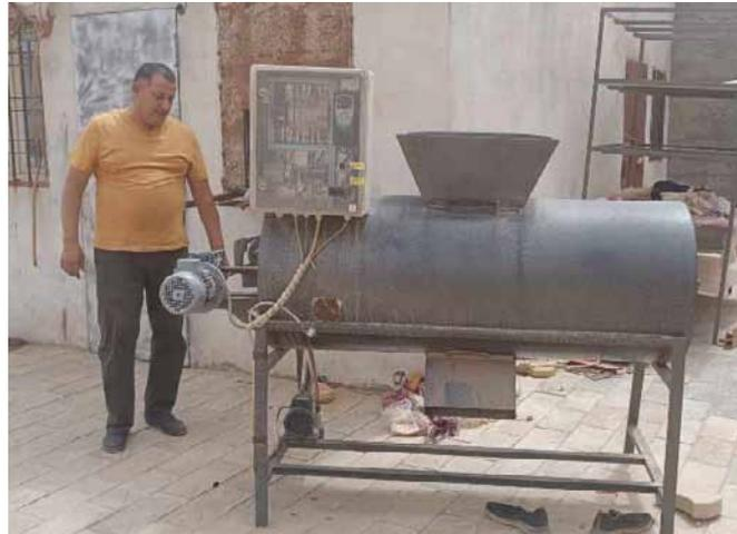
*Figure 10 : bioreactor designed for Houda Boutalbi's PhD*
